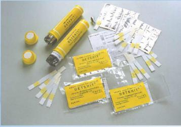
The detector strip DETEHIT<sup>®</sup> was designed for detection of nerve agents in air, water, food and on the surface. The detection strip can determine dangerous concentrations of nerve agents in the air (within 2-3 minutes), if it is possible to remove the gas mask (5-15 minutes) or whether food or water are acceptable for intake (15-30 minutes).
