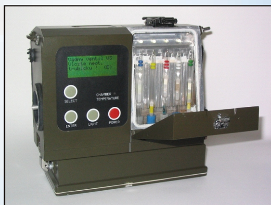
Five tubes in the new CHP-5 el. pump
