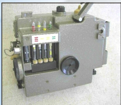
Four tubes in the CHP-71 el. pump
