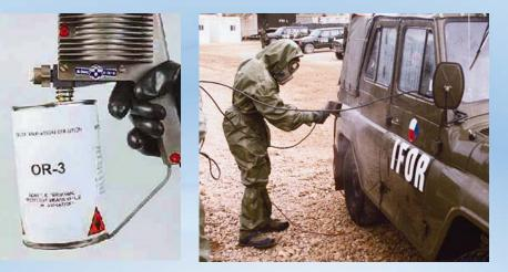
The polyvalence decontamination mixture OR-3 is intended for the decontamination of weapons and armoured fighting vehicles. It is usually applied by spraying. The OR-3 is a solution containing monoethanolamine, cyklohexylamine and potassium ethoxide.
