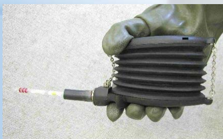
Tube DT11 in a hand pump UNIVERSAL, CZ
